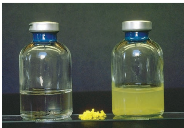
Figure 13.53 Biomining during arsenate reduction by the sulfate-reducing bacterium Desulfotomaculum auripigmentum . Left, appearance of culture bottle after inoculation. Right, following growth for two weeks and biomining of arsenic trisulfide, \text{As}_2\text{S}_3 . Center, synthetic sample of \text{As}_2\text{S}_3 .
