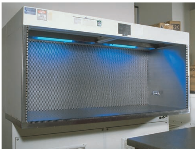
Figure 5.34 A laminar flow hood. An ultraviolet light source prevents contamination of the hood when it is not in use. When the hood is in use, air is drawn into the cabinet through a HEPA filter. The filtered air inside the cabinet is exhausted out of the cabinet, preventing contamination of the inside of the hood. The cabinet provides a contaminant-free workspace for microbial and tissue culture manipulations.
