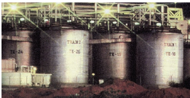
Figure 21.3 Gold bioleaching. Gold leaching tanks in Ghana (Africa). Within the tanks, a mixture of Acidithiobacillus ferrooxidans , Acidithiobacillus thiooxidans , and Leptospirillum ferrooxidans solubilizes the pyrite/arsenic mineral containing trapped gold, which releases the gold.
