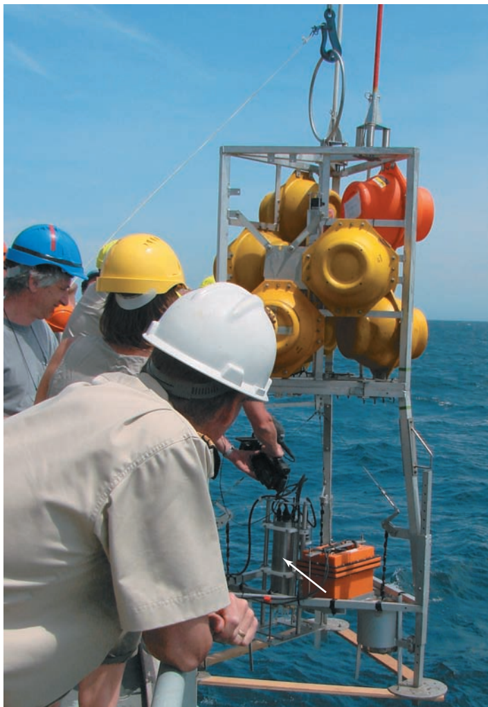
Figure 18.24 Deployment of a deep-sea lander. The lander is equipped with a bank of microsensors (arrow) to measure distribution of chemicals in marine sediments.
