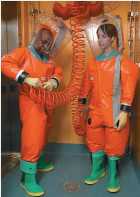
Figure 1 Biosafety level 4. Microbiologists suit up before entering the CDC BSL-4 lab. The suits supply filtered air and are positively pressurized to prevent back-flushing of laboratory air or particles.
