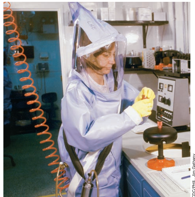
Figure 27.1 A worker in a BSL-4 (biosafety level 4) laboratory. BSL-4 is the highest level of biological control, affording maximum worker protection and pathogen containment. The worker has a whole-body sealed suit with an outside air supply and ventilation system. Air locks control all access to the laboratory. All material leaving the laboratory is autoclaved or chemically decontaminated.
